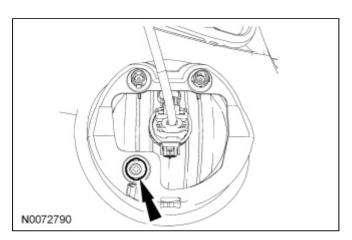
1. **NOTE:** Horizontal aim is not required for this vehicle and is not adjustable. Consult your state vehicle inspection center for recommended tolerance ranges for visual aiming.
