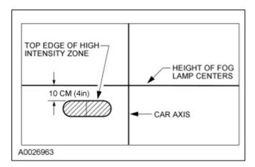
4. If necessary, rotate the adjusting screw until the fog lamp beam is within specification.
